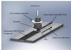
Fig.No.-3(Schematic diagram of FSP)
