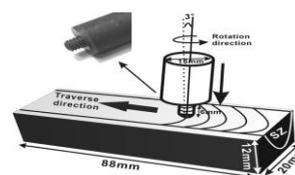
Fig no.-1 (Layout of the friction stir process)
